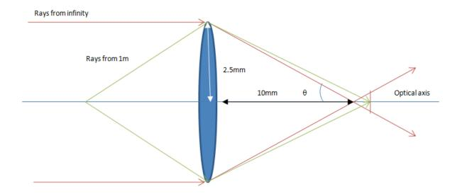
so at 10.1mm the resolution becomes  $1.342 + \tan(14.03)*100 = 26.33$  microns, which is still much larger than 3 microns, so it cannot be in focus!
