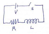
8. In the circuit shown are the same resistor, inductor, and battery of the previous problem. However, current has been flowing through the inductor and resistor for a long time. When t = 0, the switch S is closed (and the battery is removed from the circuit).
