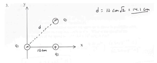
In the diagram above are three charges,  $q_1$  is at the origin;  $q_2$  is on the x-axis 10 cm away;  $q_3$  is 10 cm above  $q_2$ . The charges have the same values they have in the previous problem.
