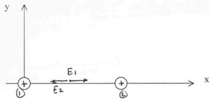
Two charges are on the x-axis. The charge at the origin is  $10 \,\mu\text{C}$ ; the second charge,  $10.0 \,\text{cm}$  away, is  $20 \,\mu\text{C}$ .
