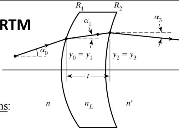
The *RTM* for a thick lens:
